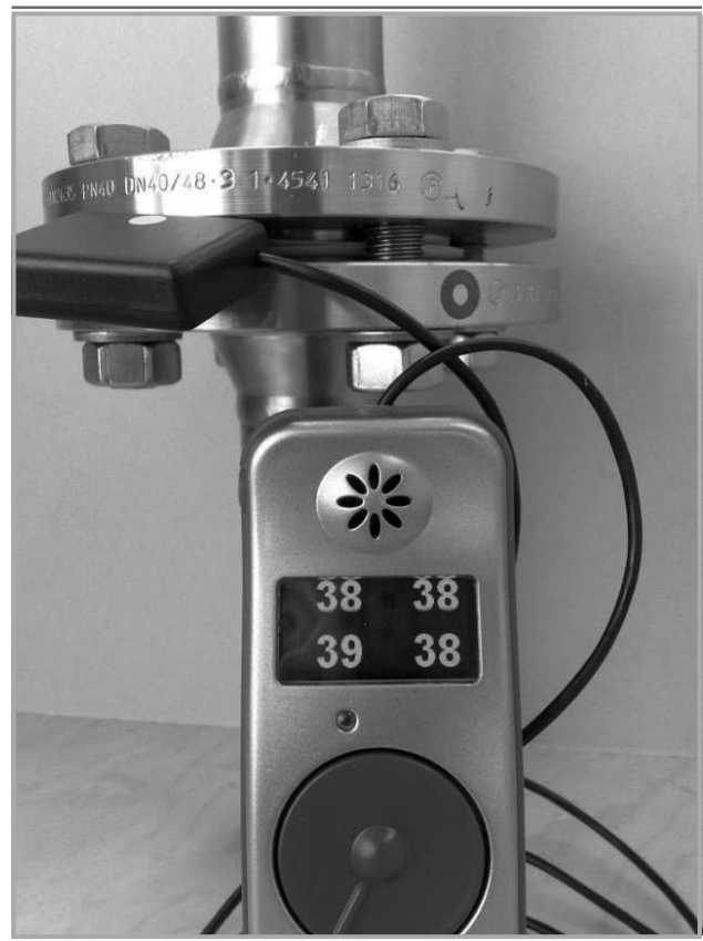
KCS handheld, surface pressure in 4 partitions. Gasket profile PW 21i; flange DN 40 PN 40
